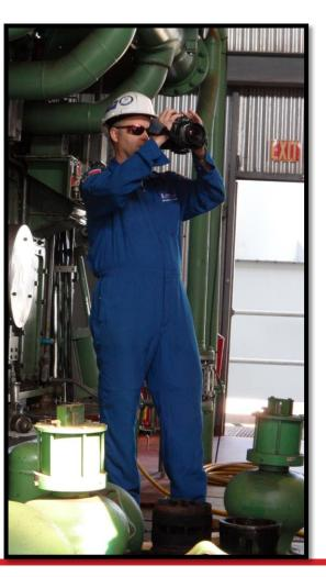
Opgal's EyeCGas<sup>®</sup> is an innovative Optical Gas Imaging (OGI) camera For detection of hydrocarbon gasses.
